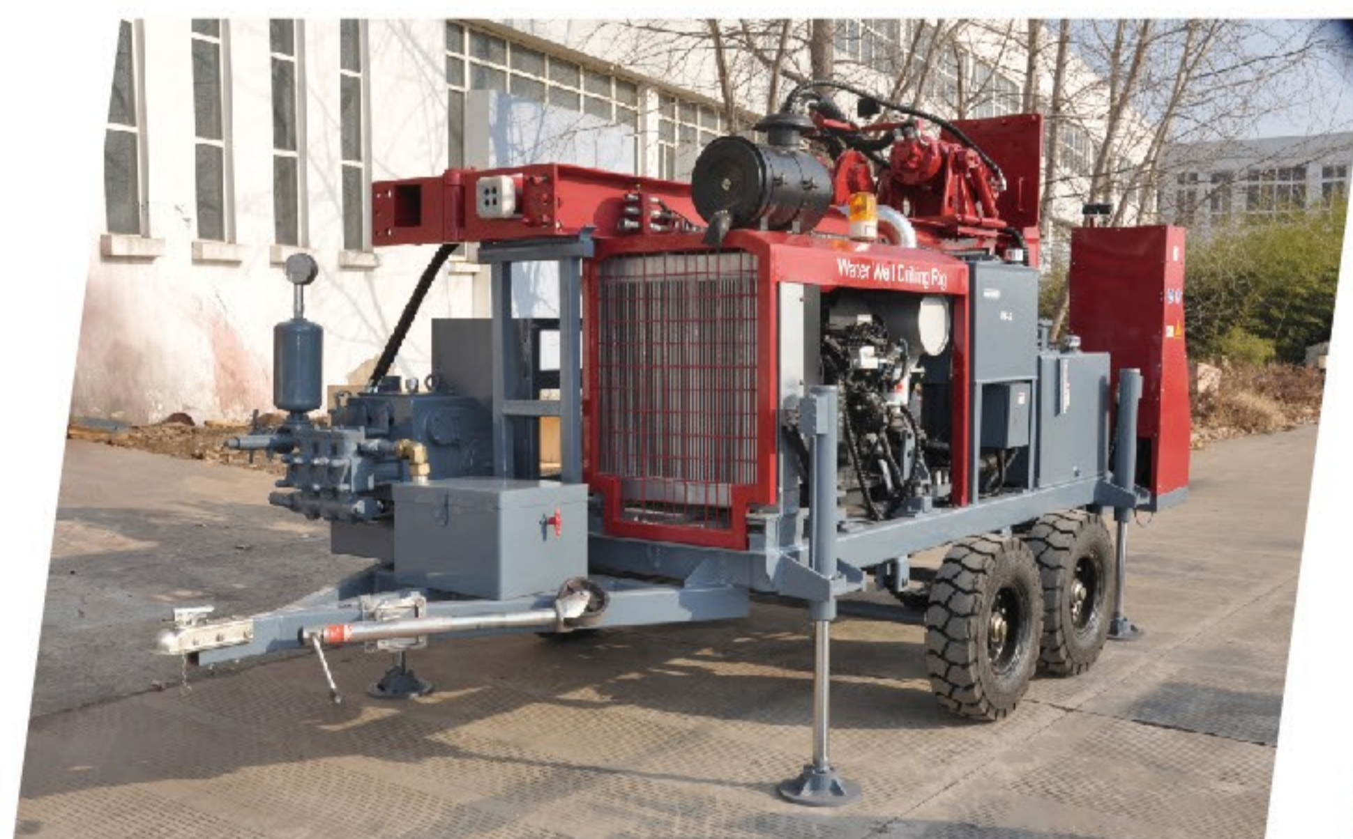
Fold mast, possible to lift 6 m length drill rod
