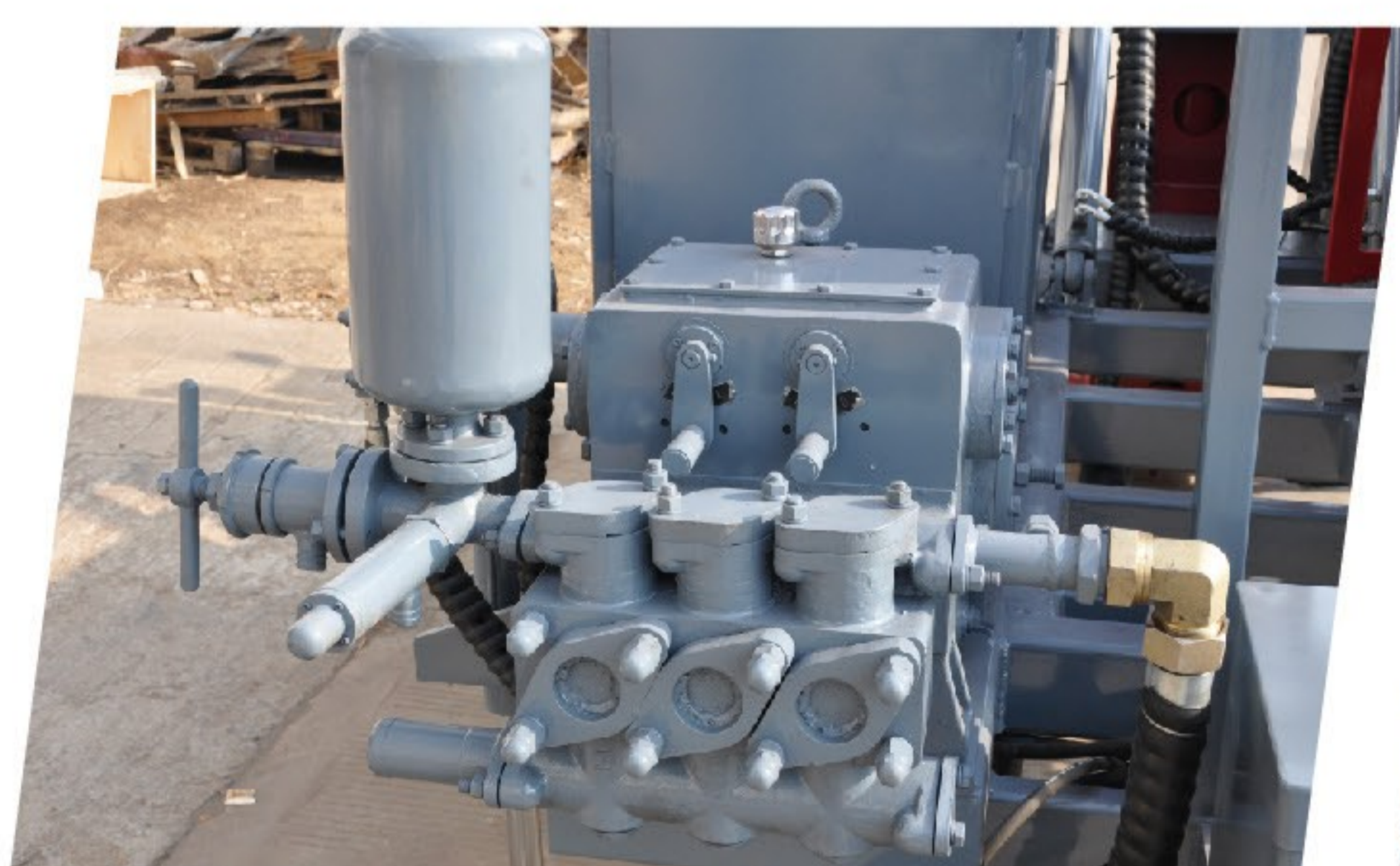
The mud pump be equipped, also air compressor also be chose.
