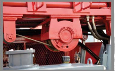
The capacity of hoist is 2 ton.
