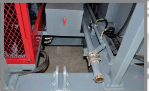
Open/close of drilling fluid supply is controlled by hydraulic cylinder.
