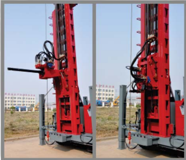
Adjusting angle of mast 0-90° Easy to load the drill rod
