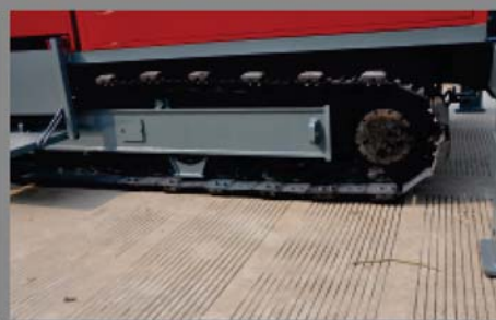
Standard excavator chassis with South Korea imported drive motor increase the flotation of drill rig. Can be equipped with rubber track.
