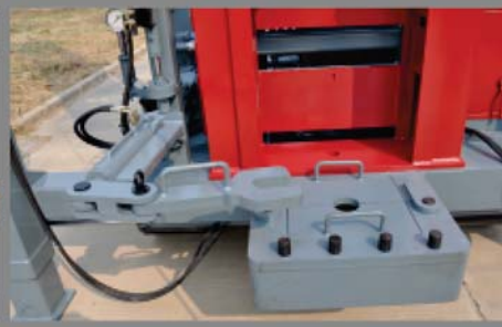
Clamping system can be adjusted for height
