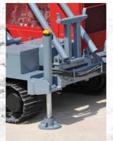
The telescopic mast ensures the reliability of drilling. The underside end of the drilling mast anchors the ground surface while drilling, providing additional stability. While transportation mast can be moved to center of gravity of the rig for more safety.
