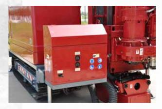
The operator panel is equipped with non-fixing control joysticks, which provide additional safety for the operator. Drilling and rotation joystick with friction damper and non-fixing hoist joystick provide convenience and safe operation. There is auto alarm function forlow level of hydraulic oil.
