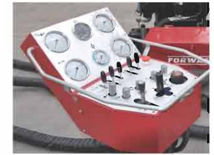
The pilot hydraulic control system provides the operator with full control. The operator station works at a reduced hydraulic pressure (max 80 bar) which means it's safer for the operator and lighter in weight.
