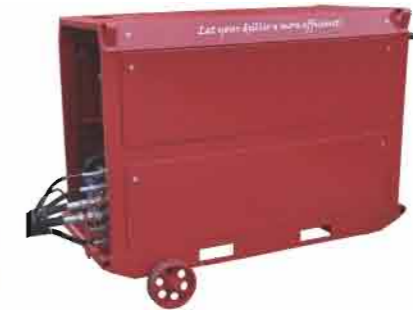
Drilling time is maximized by the electrical power units and cleverly designed hose arrangements which feature a hose ladder to reduce wear.
